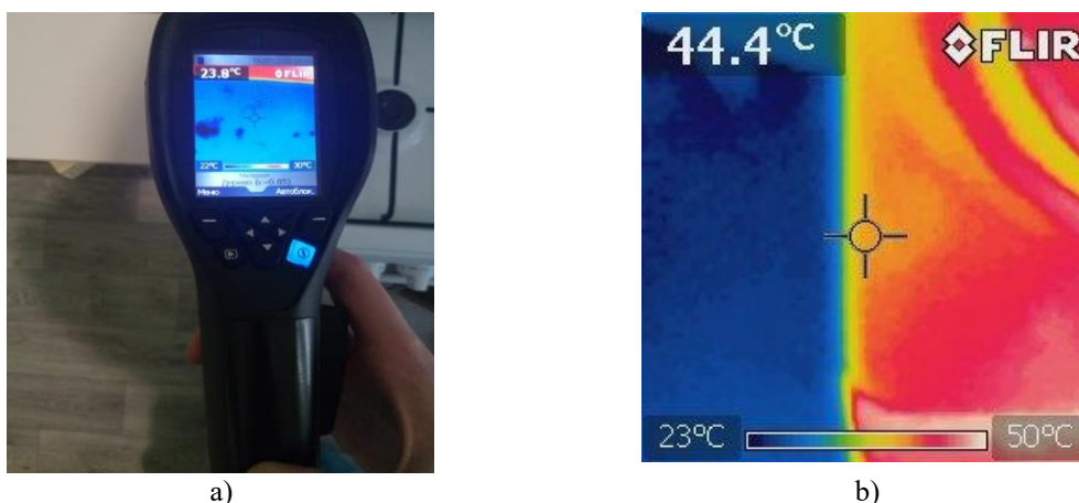
Fig. 6 Sample of kitchen countertop during determining its temperature: a) the sample temperature at the limit of "cooking surface - countertop" at the beginning of heating; b) sample temperature at the limit of "cooking surface - countertop" after 1 hour of oven and cooking hobs working.
