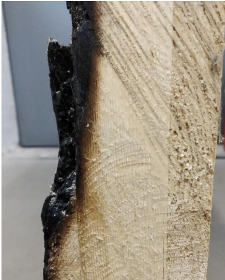
Fig. 3 Cross-section of the sample after the medium-scale test.
