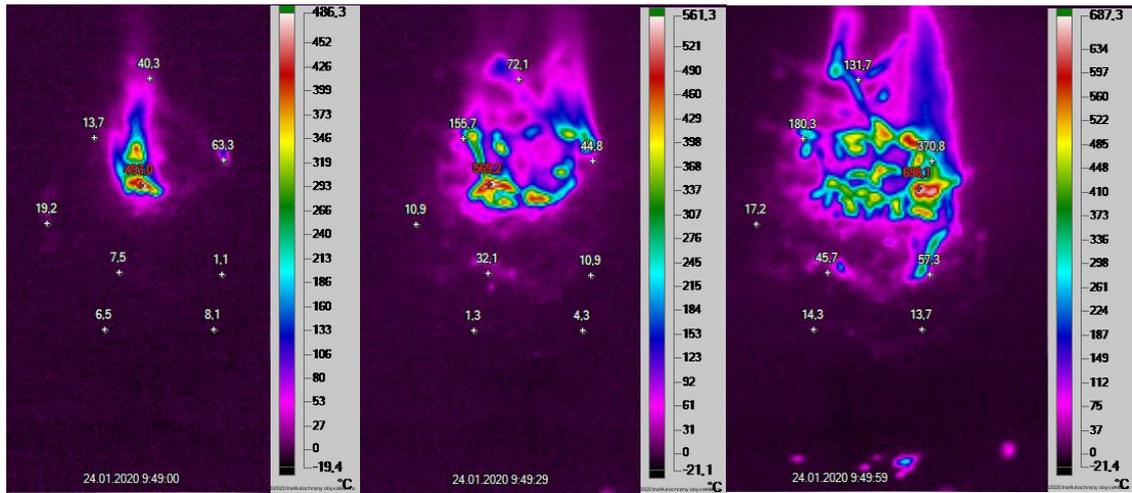
Fig. 8a, 8b,8c - Experiment no. 4 – Spreading of the fire at 30 seconds, 60 seconds, 90 seconds.
