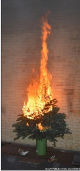
Fig. 4 Experiment no. 2 - The spreading fire at 210 seconds
