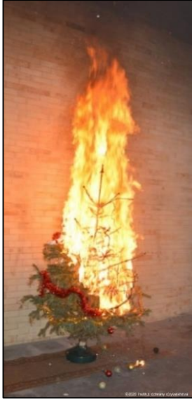
Fig. 5 - Experiment no. 4 – Spreading of the fire at 150 seconds
