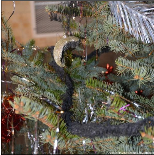
Fig. 7 Experiment no. 3 – View of the burned garland and a partially burned ornament
