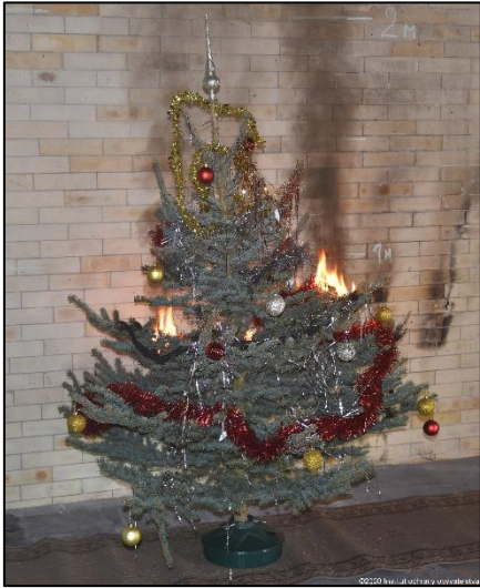
Fig. 6 Experiment no. 3 – Spreading of flames on the Christmas garland
