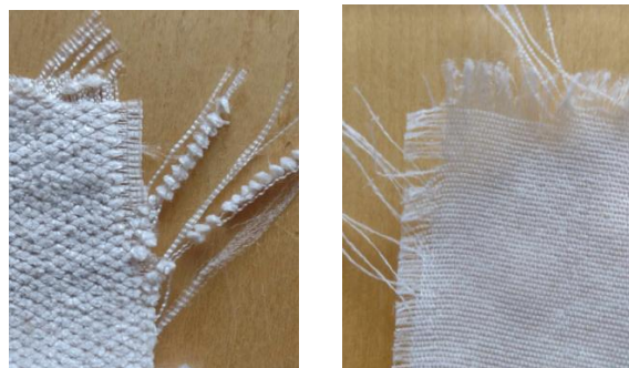
Fig. 1 Structure of upholstery fabric LONDON : (a) face side, (b) back side.
