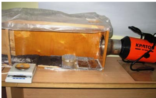
Fig. 1 The laboratory stand for blowing off of a dispersive material.
