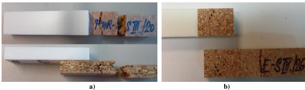
Fig. 4 Damage to glued joint using plastic + PB at the humidity WR 45% a) PUR adhesive , b) epoxy adhesive
