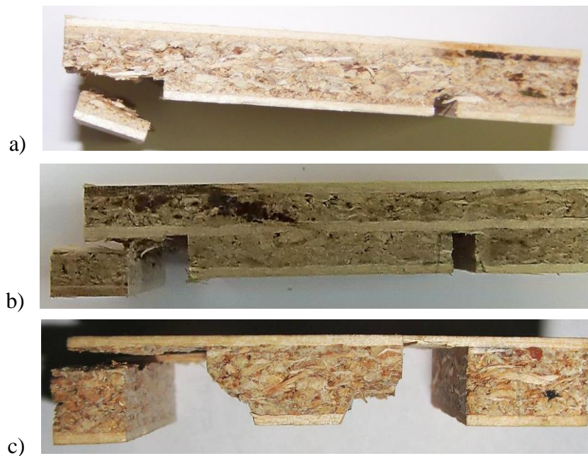
Fig. 6 The typical chipping fractures of the samples: a) assembly diagram No 1a; b) assembly diagram No 3; c) assembly diagram No 4.
