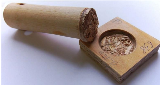
Fig. 5 . The typical plywood sample fracture in response to cleavage.
