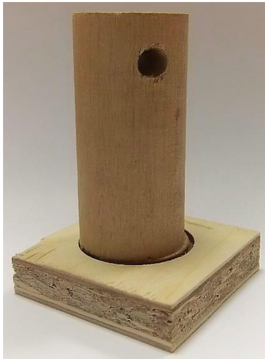
Fig. 1 The image of the sample to determine the surface soundness.
