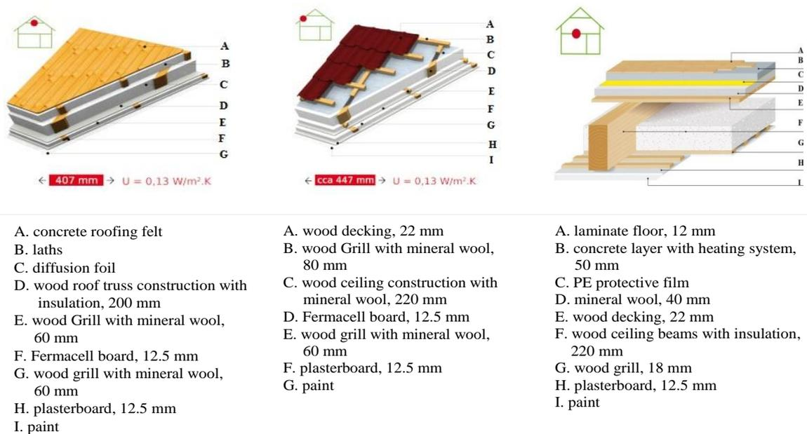
**Fig. 4 Components of roof and ceiling for the Reference Prototype Building.**
