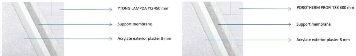
**Fig. 2 Components of exterior walls for alternatives A1-A2.**
