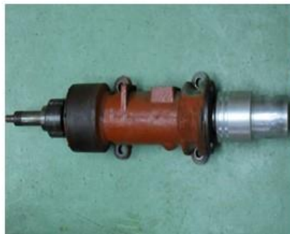
Fig. 4 Spindle and its bearings.
