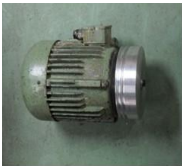
Fig. 3 Electric motor with a pulley.
