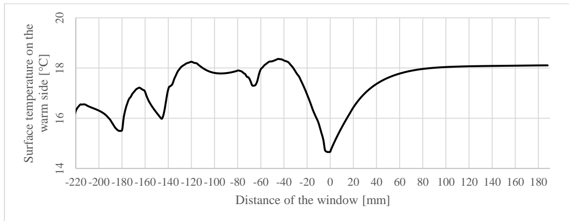
Fig. 2 Interior surface temperature of the wooden window frame and IGU whit Chromatek ultra F spacers - detailed model. \theta_{si \text{ min}} = 14.65^\circ\text{C} .
