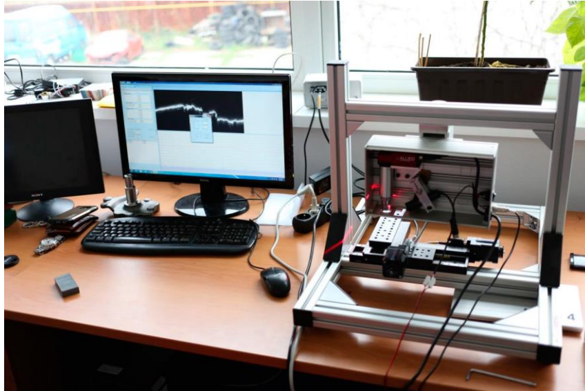
Fig. 4 Laser profilometer during experimental measurements ready for exchange of the laser light source.
