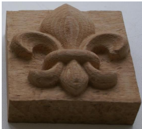
Fig. 4 Product “rose” after finishing 3D-milling and manual finish; beechwood, planned dimensions – 80 × 80 mm (a), the maximum relief height – 25 mm.
