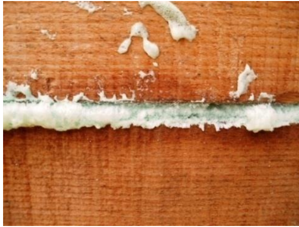
Fig. 12 Unexposed side of their test sample with the flammable PUR foam after thermal loading for 60 min.
