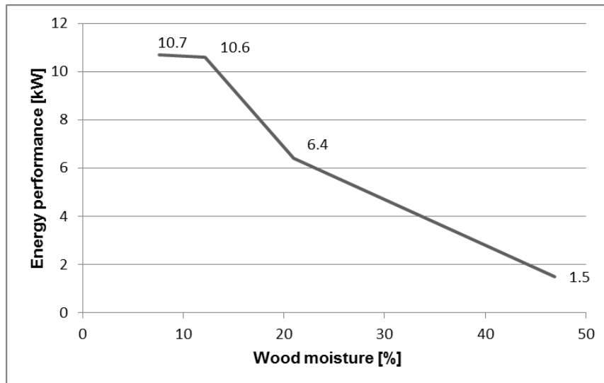
Fig. 4 The effect of wood moisture content on the energy performance of the fireplace insert.
