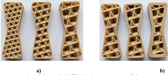
Fig. 2 Visual representation of the analyzed 3D printing parameters of the connectors: (a) cubic infill densities of 40%, 30%, and 20% (from left to right); (b) number of perimeters, perimeter thickness corresponding to 1P, 3P, and 5P (from left to right).
