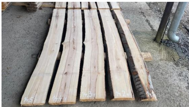
Fig. 2 Labelling of sawn timber from a beech log prior to CT scanning
