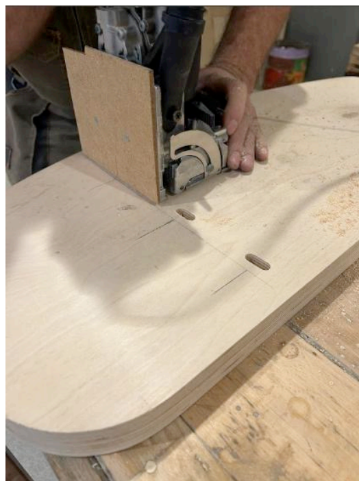
Obr. 4 Výroba otvorov na spoje Fig.4 Creating holes for joints
