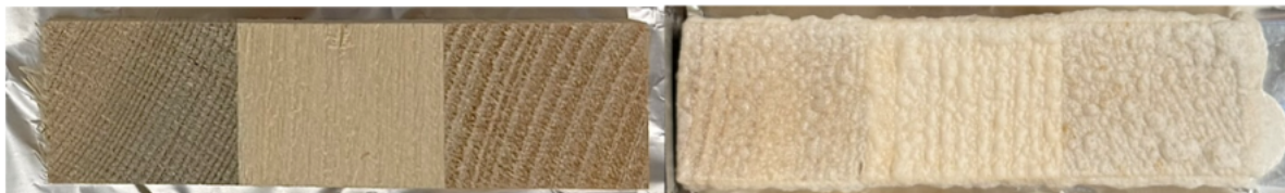
Obr. 2 Porovnanie neošetrenej a ošetrenej vzorky pri teplote 100 °C na konci merania Fig. 2 Comparison of non-treated and treated sample at 100 °C at the end of measurement
