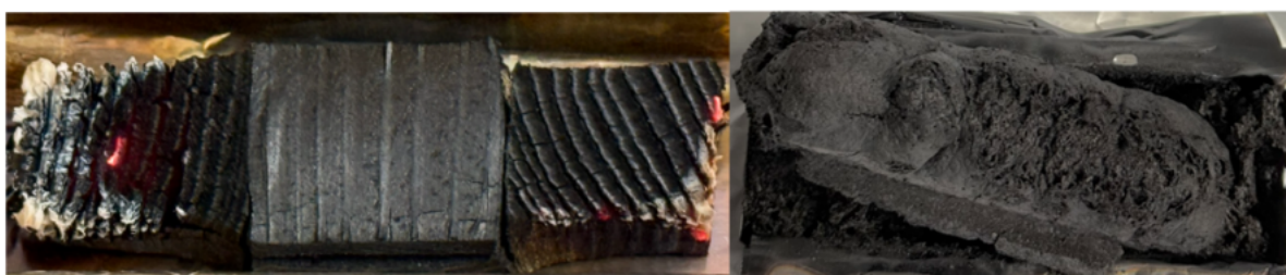
Obr. 5 Porovnanie neošetrenej a ošetrenej vzorky pri teplote 250 °C na konci merania Fig. 5 Comparison of non-treated and treated sample at 250 °C at the end of measurement
