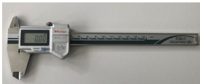
Fig. 4 Measuring device for determining yarn slippage (authors' archive)
