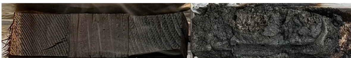
Obr. 4 Porovnanie neošetrenej a ošetrenej vzorky pri teplote 200 °C na konci merania Fig. 4 Comparison of non-treated and treated sample at 200 °C at the end of measurement
